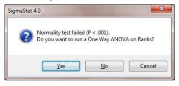
SigmaStat automatically checks your data against the underlying assumptions for normality, equal variance, and multicollinearity. SigmaStat warns you of violations and suggests a more appropriate test when necessary.
